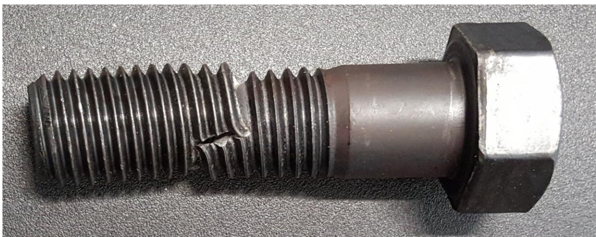
Figure B.4 Tension failure
