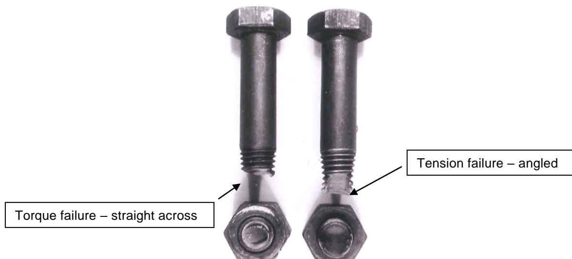
Figure B.1 Torque and tension failure mode surfaces
