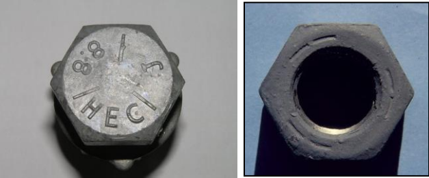
(a) AS/NZS 1252.1 property class 8.8 bolt assembly components
