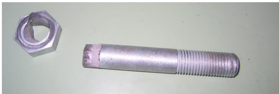
Figure B.6 Bolt head breakage
