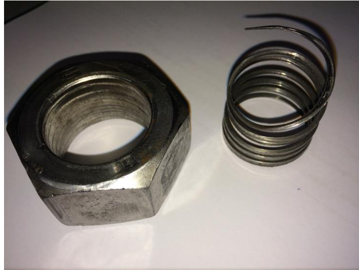
Figure B.5 Thread stripping failure
