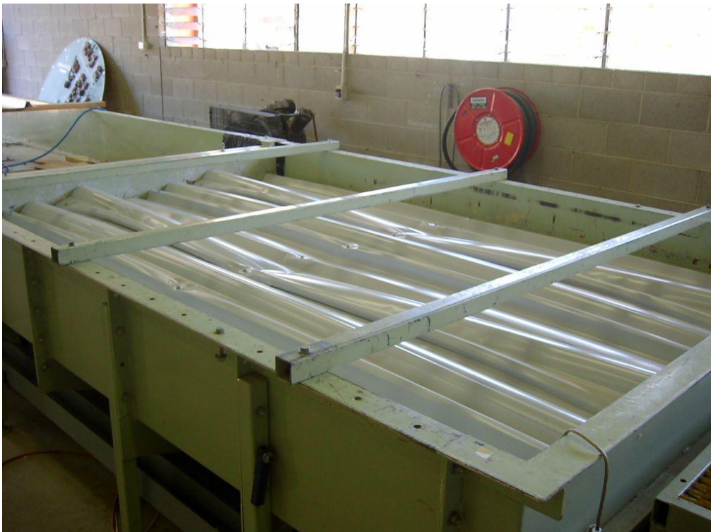
Low-High-Low testing at JCU Cyclone Testing Station, Townsville QLD
