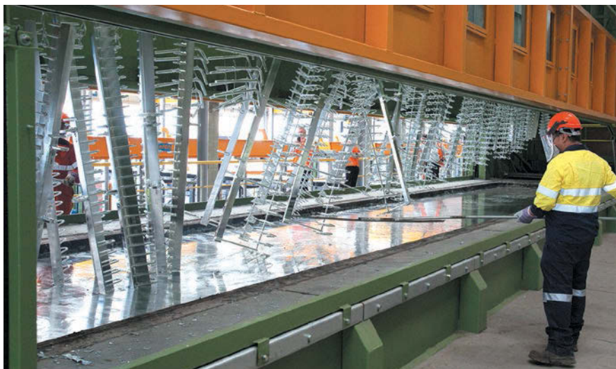
Sweeping as articles are lifted from the kettle at the Kewdale facility to remove zinc oxide by-product to ensure a smooth quality finish.
