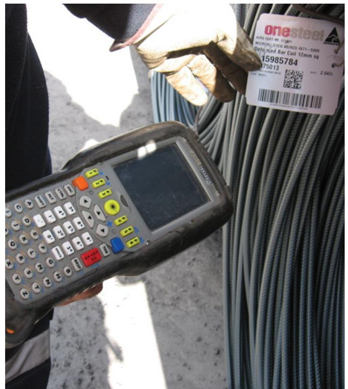
A warehouse operator at Laverton scans a coil of 12mm deformed reinforcing bar using the mobile scanning device. The 'OneTag' label clearly shows all the relevant product information and two barcodes being printed – the GS1-128 barcode and the GS1-DataMatrix with clear reference to ACRS Certification.
