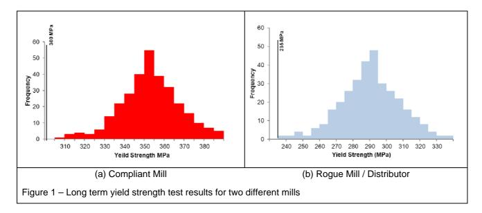
The compliant mill (Figure 1(a)) targets a mean yield strength value well above the minimum requirement of AS/NZS 3679.1 300 Grade. Obviously some of this material will be above the average and some below the targeted average, however all batch test results will be above the 300 MPa minimum.
