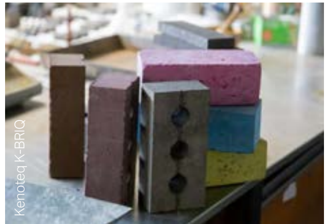
Figure 78: Bricks made from up-cycled construction waste and a lower temperature firing process
