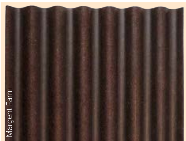
Figure 93: Example of hemp corrugated sheet
