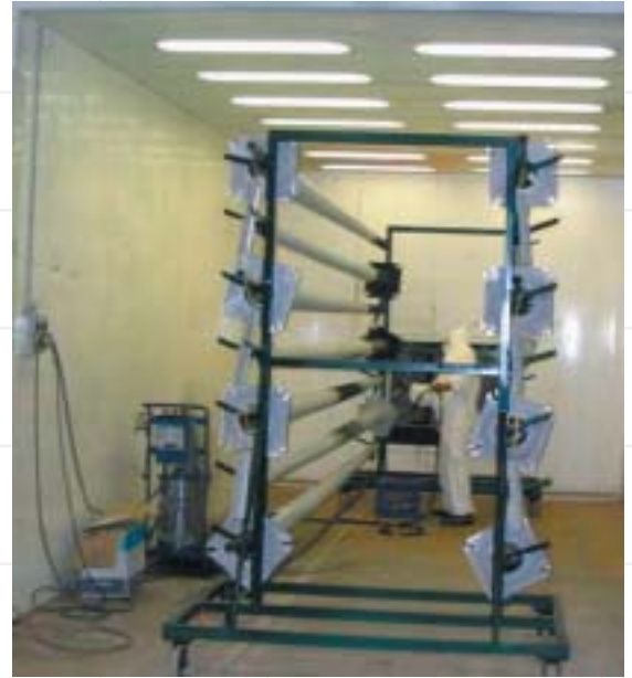
Superior Coaters uses a batch powder coating system for coating all of INGAL EPS' Estate Poles. On-site garnet blasting facilities and large booths and ovens allow the processing of these larger galvanized poles.
