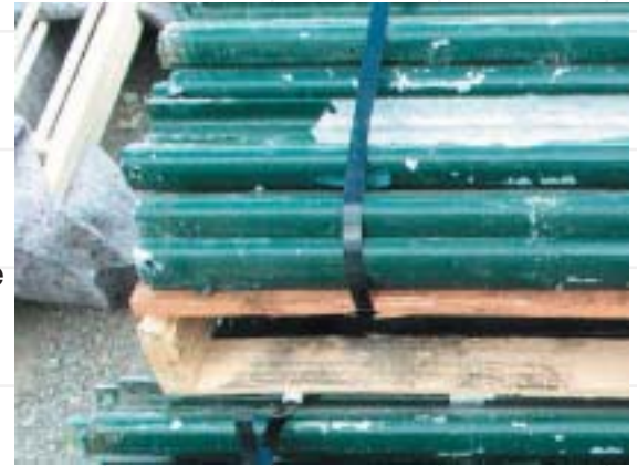
Poor pre-treatment resulted in this total failure of the polyester powder coating in these galvanized posts.
