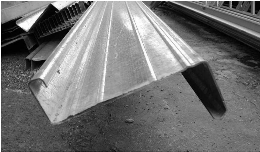
Fig. 1.2 Innovative SupaZed™ section
