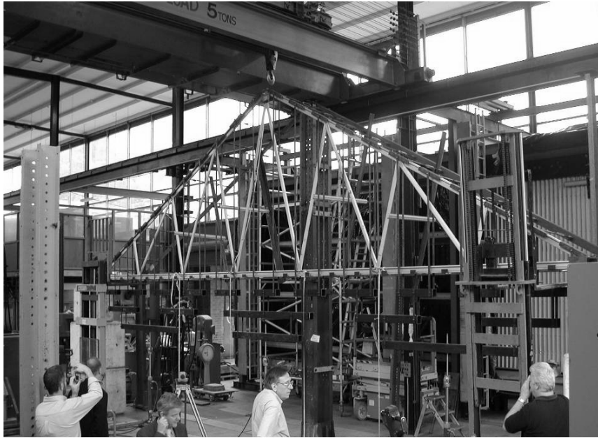
Fig. 1.9 Roof truss under test
