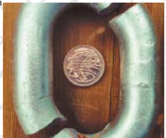
Hydrogen embrittlement failure of Herculloy chain is caused by exposing this 1200 MPa steel to pickling acid. These types of steels should not be galvanized.
