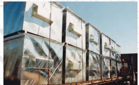
Thin, flat sheet will always buckle in the galvanizing process. Corrugating or ribbing of these type of sections will significantly reduce the likelihood of distortion during galvanizing.
