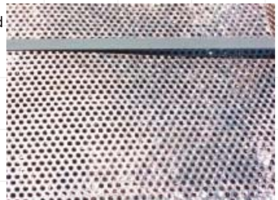
Blinding of small holes (6mm or under) will occur because of the surface tension of the molten zinc. This can be minimised by detailed attention to the item as it emerges from the molten zinc.
