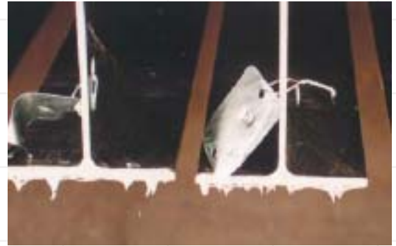
Drainage spikes will always occur where edges are parallel to the molten zinc surface. These are removed by grinding or filing during the inspection process.
