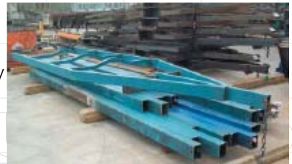
While the primer used on pipe sections is designed to easily removed in the galvanizers' pre-treatment process, uncoated sections (at the back) are much faster to process as they do not require paint stripping.
