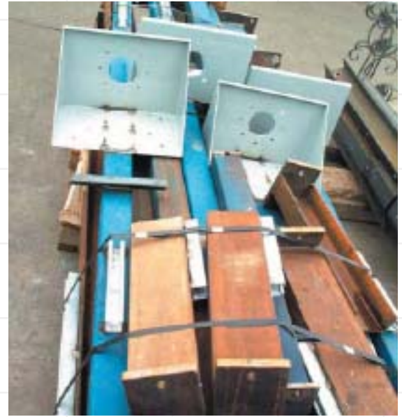
This load of fabricated steel contains a mixture of black steel, galvanized steel, painted and powder coated components welded in assemblies. This causes problems in the pre-treatment process for galvanizers
